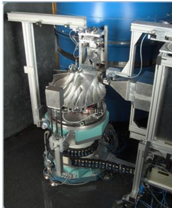
Fig. 1. The dedicated residual stress instrument StressSpec at the research reactor FRM II in Garching, Germany, with a huge impeller on the sample table.
