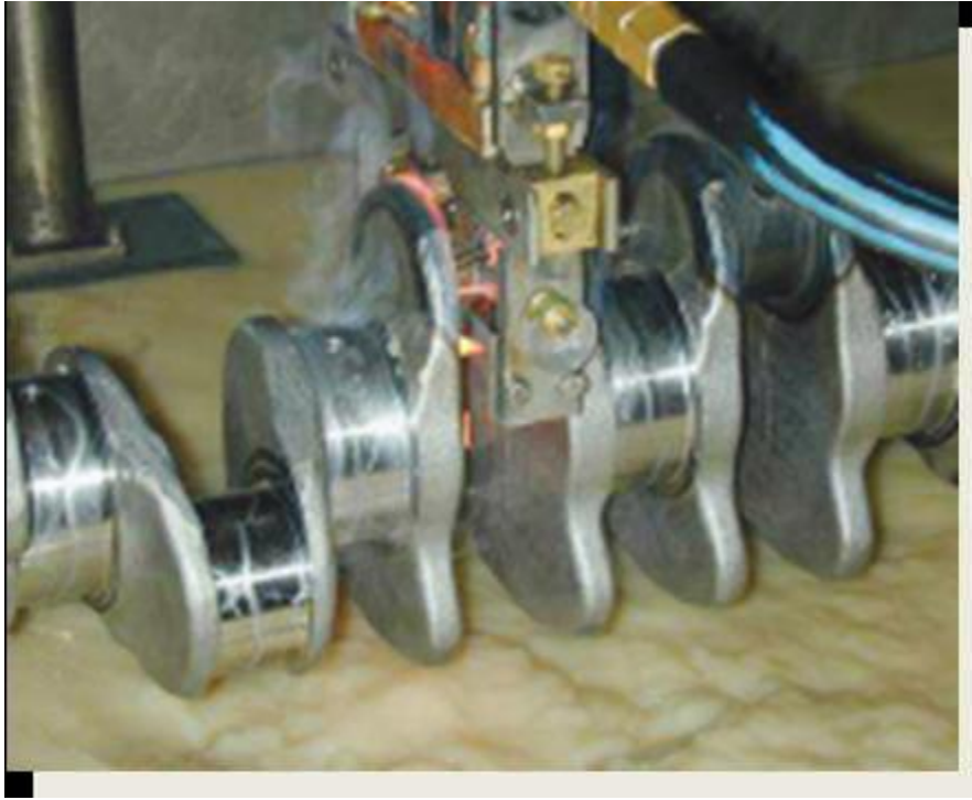
Fig. 2. Induction hardening of a con-rod bearing of a truck crankshaft.
